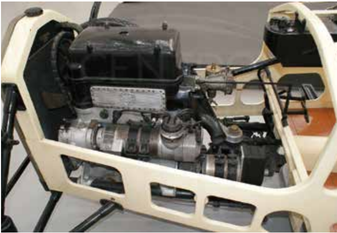
Fig. 8.5. Arrangement of the power unit on the unitised body (National Automobile Museum).
