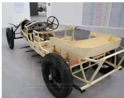
Fig. 8.4. Structure of the unitised body of the Lambda (National Automobile Museum).
