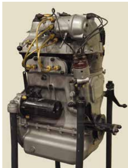
Fig. 11.9. Prototype Aprilia engine, with indirect injection (Lancia Collection).
