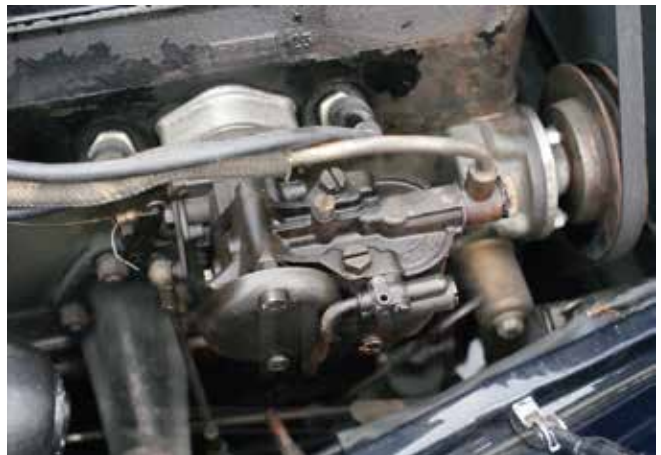
Fig. 10.18. Detail of the carburettor of the Augusta (Gallery of Historic Locomotion, Rivarolo Canavese).
