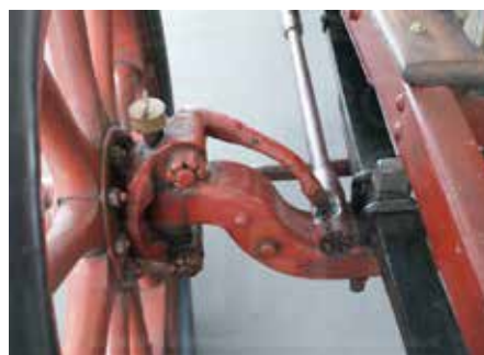
Fig. 3.8. Detail of the front axle with nailed curved element (National Automobile Museum).
