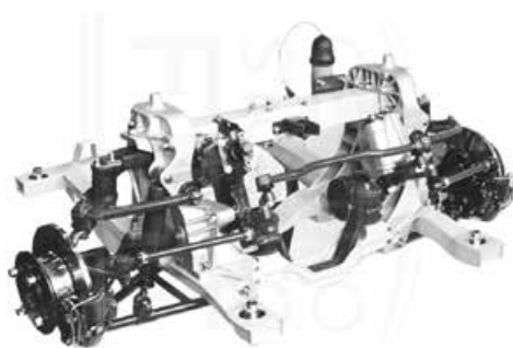
Fig. 14.18. Subframe and front suspension of the Flavia (FIAT History Centre).
