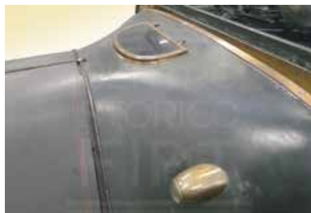
Fig. 6.6. Skylight for the instrument panel of the 35 HP/Theta Coupé de Ville (Lancia Collection).
