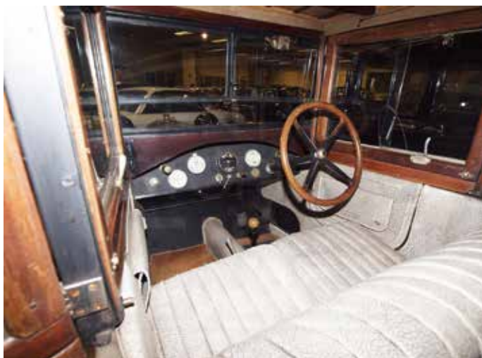
Fig. 8.17. Interior of the Lambda Berlina; the lengthwise-sliding side windows should be noted (Lancia Collection).
