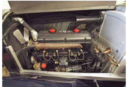
Fig. 8.25. External view of the compact 8 cylinder Dilambda engine (Lancia Collection).
