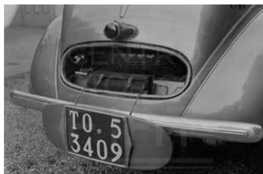
Fig. 11.14. Detail of the spare wheel compartment of the Ardea I series (FIAT History Centre).
