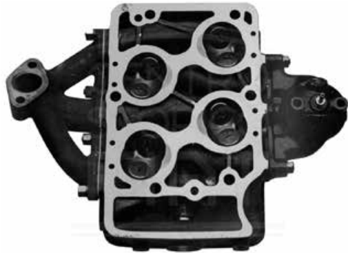
Fig. 11.18. Arrangement of the valves in the Ardea engine (FIAT History Centre).
