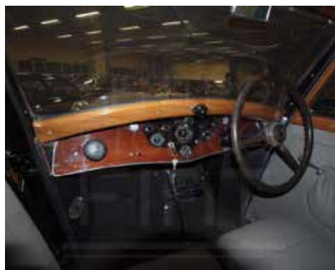
Fig. 9.16. Dashboard with shock absorber control of the Lancia Astura Berlina III series, bodywork by Carrozzeria Castagna (Lancia Collection).
